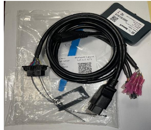
The cables have a male, female port and gateway connector.
