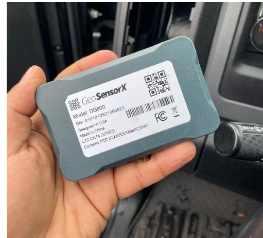
Locate Serial Number. Each Gateway (and Dash Cam) have been pre-assigned to a specific vehicle and must be installed in that vehicle only.
