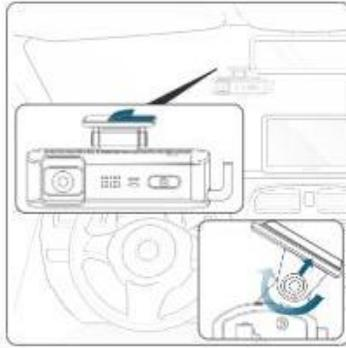
Completely remove the protective sheet from the mounting tape. Permanently attach the DC400 AI Dash Cam to the windshield at the identified location. Then tighten screw on the mount using the Allen key.
