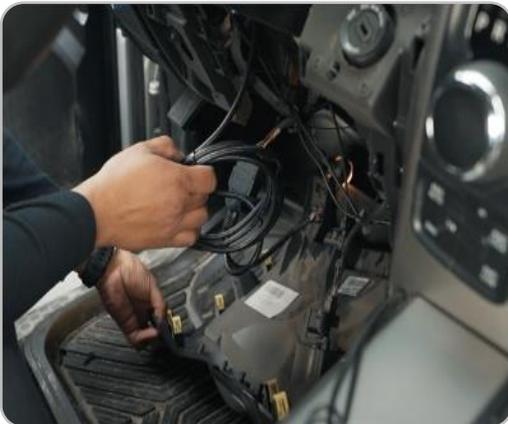
Connect the Gateway Connector into the Gateway
