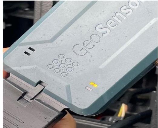
Power on the device. During the boot up process the device will flash Orange and Green for 1 second and then go off. This represents the device powering up.
