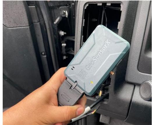
Connect the Gateway Connector into the Gateway
