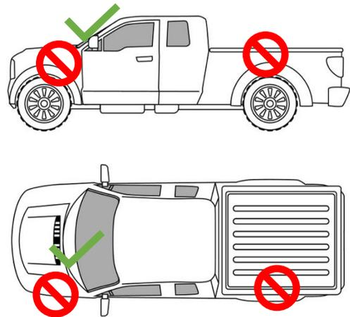
**DO NOT** install the unit underneath metal as the signal will not penetrate and reach the satellite.
