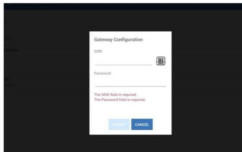
Go to "Gateway Configuration", in this tab is where you will enter the VG800's SSID.
