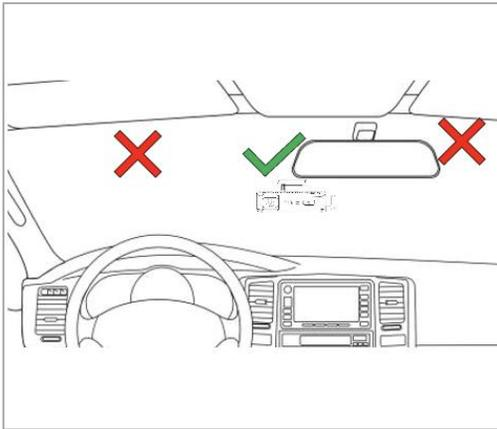
Start by cleaning the area of where you are placing the Alcam400. Our recommended location on the windshield will be to the left of the Rear View Mirror within the Wiper Path. (Reference diagram A)
