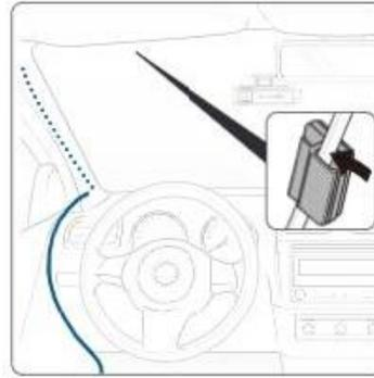
Run cable across top of windshield. Secure using cable clip or tuck cable under glass seal around windshield.
