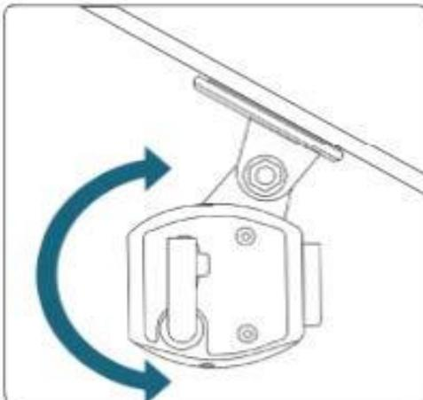
Adjust camera angle so that it hangs perfectly vertical.
