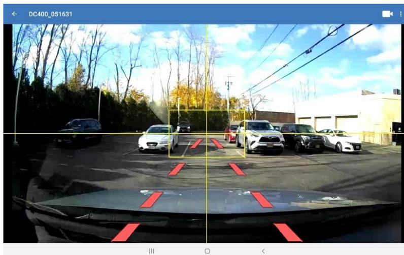
Make sure the grid on the screen has the road view on the bottom half, and the horizon on the top half.
