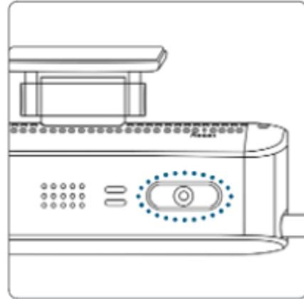
Press and hold the panic button next to the Driver Camera Lens for approximately 5-7 seconds until you hear a chime. This enables the WIFI function on the Alcam400.
